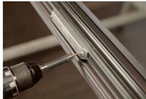
Direct punching of the tie rod
